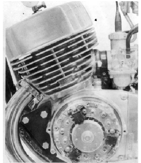
Use a dial gauge on an H1D or H2 model ignition system to align the pointer with the L mark for the left cylinder, the C mark for the center cylinder, and the R mark for the right cylinder. Then align the pointer with each of the S marks to position the signal coils. Be sure to go through the entire timing procedure for each signal coil before doing another.
