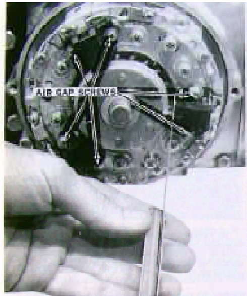
Always adjust the air gap of all three signal coils on H1D and H1E models. Loosen the screws noted above to move the signal coils. CAUTION: Do not pry on the signal coils with any kind of tool or they will break.
