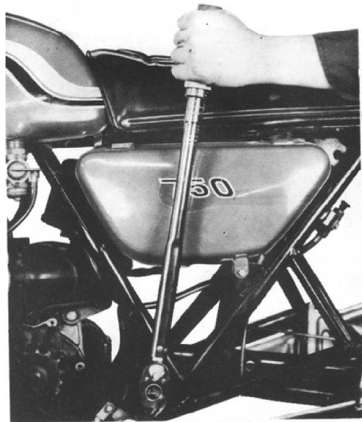
Tighten the swingarm pivot bolt with a torque wrench to the specifications mentioned in the accompanying text. If the swingarm is loose, the motorcycle will not handle properly. If it is too tight, the pivot will bind and give the motorcycle a rough ride.
