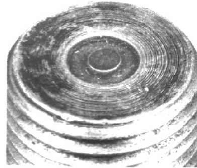
Low-temperature fouling. The soft, sooty deposits indicate incomplete combustion. Possible causes are rich carburetion, weak ignition, retarded timing, or low compression.
