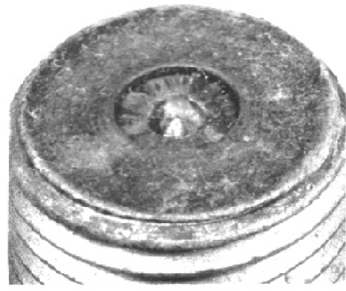
Worn-out spark plug. This amount of electrode wear can cause misfiring during acceleration or hard starting.
