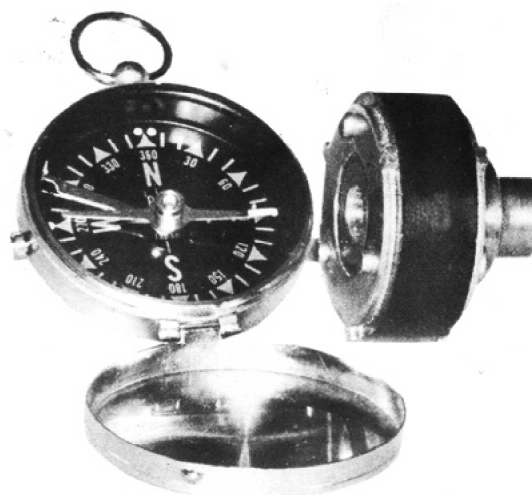
To check for a reversed magnet in the signal rotor, hold a compass near the rotor, then move it around the face of the rotor. If the needle swings around end-for-end, it indicates a reversed magnet.
