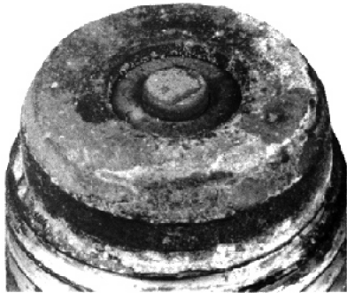
Normal spark plug. The deposits are light tan or gray, indicating good engine and ignition system conditions. The electrode wear indicates normal spark rotation.
