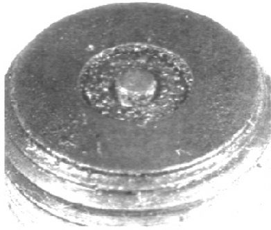
Cold-foul spark plug. These wet fuel/oil deposits can be caused by "drowning" the spark plug with raw fuel during cranking, an excessively rich fuel/air mixture, or a weak ignition system.
